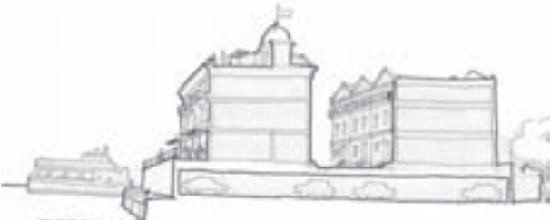
An early section drawing of the ferry district buildings showing how the parking structure helps to elevate the public buildings putting them out of flood levels.
